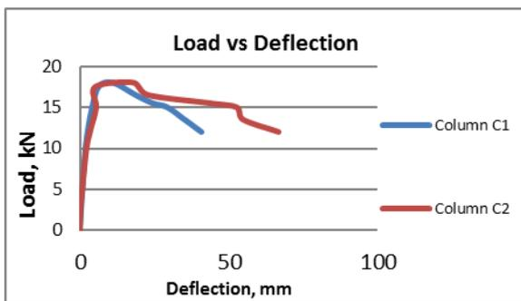
**Fig. 11(b): Load-Deflection behavior of column C<sub>1</sub> and column C<sub>2</sub>**
