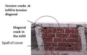
**Fig. 12(h): Diagonal crack at infill in the final stage and spalling of concrete in beams and spalling of infill**
