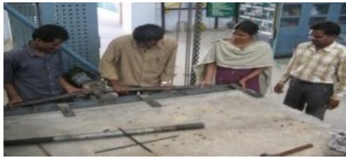
Fig .2: Fixing of loading frame
