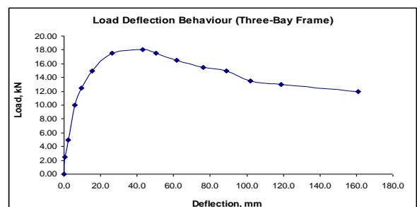
Fig. 3(b): Base shear vs storey deflection of three-Bay frame (Back-Bone Curve)
