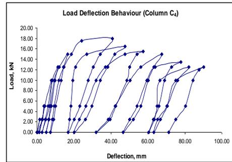
Fig. 6(a): Base shear vs. storey deflection of column C4
