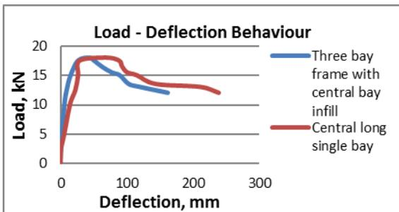
**Fig. 11(a): Load-Deflection behavior of three bay frame and single long bay frame**
