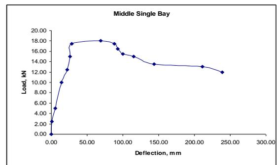
Fig. 4(b): Base shear vs storey deflection of middle long single-Bay frame (Back Bone-Curve)
