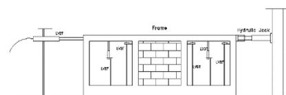
Fig. 1(c): Schematic diagram of test set-up (Side View)
