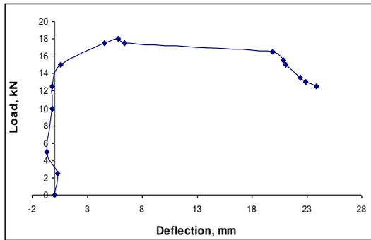
**Fig. 10(b): Lateral load vs. vertical deflection of slab middle with beams (Back-Bone Curve)**
