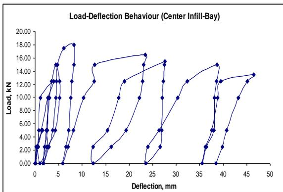
Fig. 5(a): Base shear Vs storey deflection of infill bay
