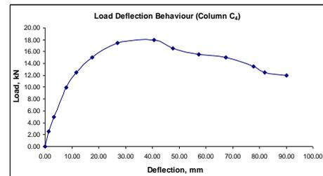
Fig. 6(b): Base shear vs. storey Deflection of column C4 (Back-Bone Curve)
