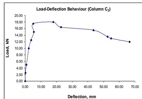
Fig. 8(b): Base shear Vs storey deflection of column C<sub>2</sub> (Back-Bone Curve)
