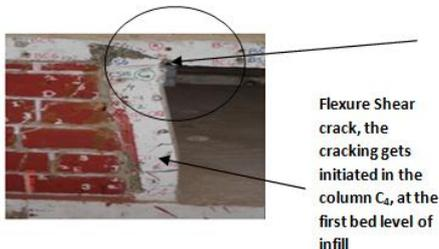
**Fig. 12(e): Flexure shear crack in column C4, crack in C4-B1-B5 Joint and spalling of CONCRETE**
