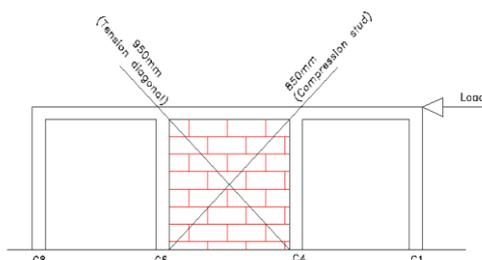
**Fig. 12(i): Diagonals in tension and contraction of infill in the final stage**
