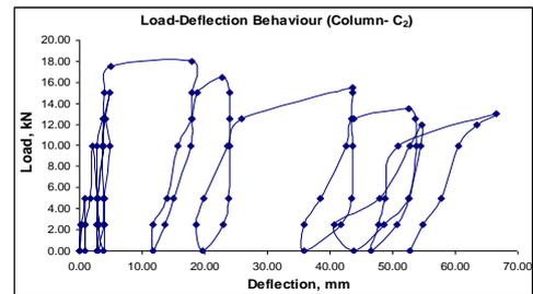
Fig. 8(a): Base shear Vs storey deflection of column C<sub>2</sub>
