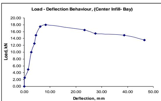
Fig. 5(b): Base shear Vs storey deflection of infill-bay (Back-Bone Curve)
