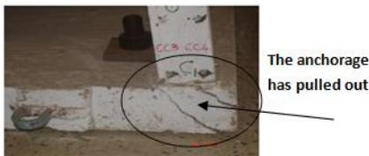
**Fig. 12(f): Cracks in foundation-Column C1 joint**
