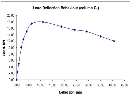
Fig. 7(b): Base shear Vs storey deflection of column C<sub>1</sub> (Back-Bone Curve)
