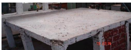
**Fig. 9: RCC Slab in Three-Dimensional Frame**
