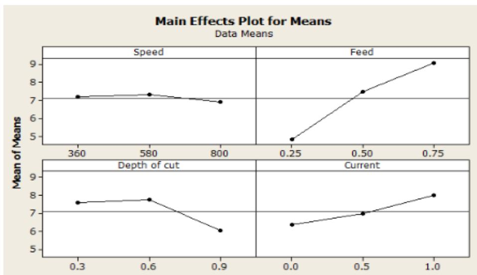
**Fig. 5: Main effects for surface finish ( $R_a$ )**
