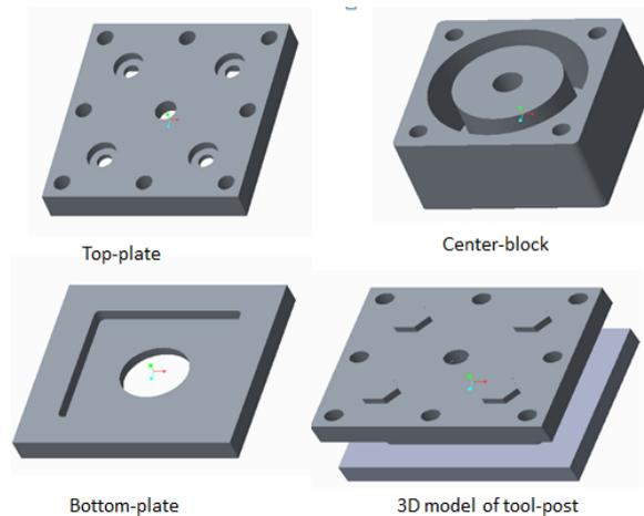
**Fig. 2: 3-D views of individual and assembled parts of proposed tool-post**
