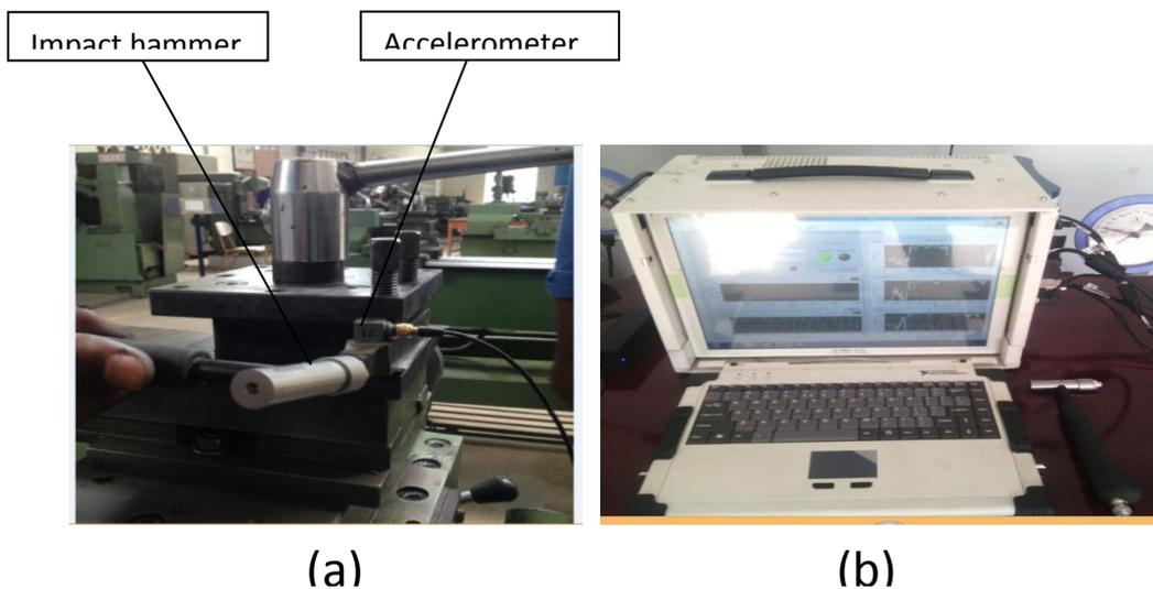
**Fig. 3: Tool-post and acquisition of vibration signals (a) Hitting of impact hammer in axial direction. (b) Interfacing of accelerometer and impact hammer with PXIe-4496**
