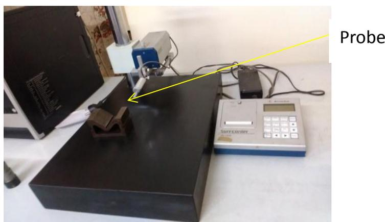
**Fig. 4 SURFCORDER SE-1200 surface measurement instrument with interface**
