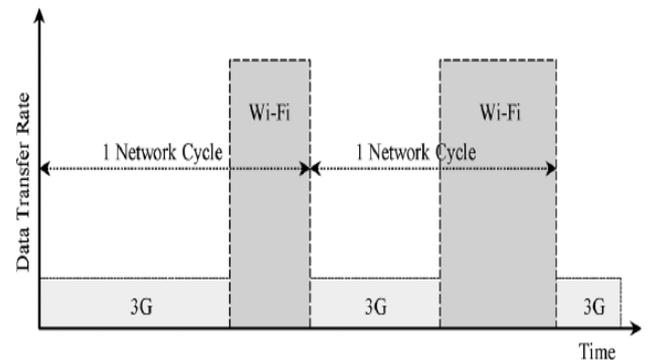
Figure 1: An Example of using Both 3G and Wi-Fi to Transfer Data
