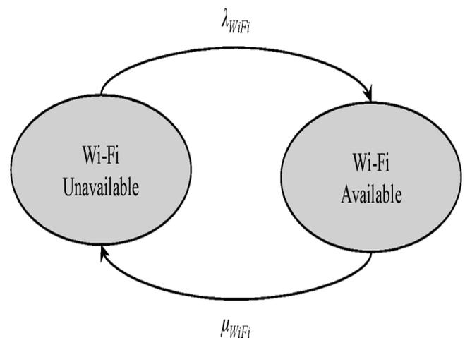
Figure 2: State Diagram of a Wi-Fi Network
