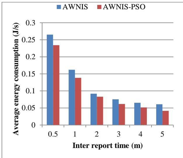
**Fig. 8: Average energy consumption and delay comparison (I) between Awnis and Awnis-PSO with the ECG Workload, where the number of APs is 15. (a) Average energy consumption according to the inter-report time**
