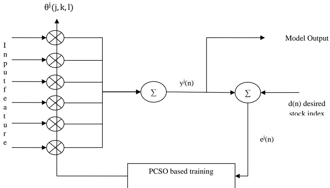
Figure 3: Adaptive Linear Model
