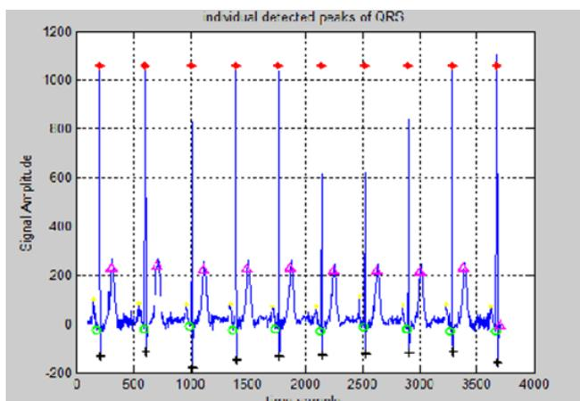
Figure 14: QRS detected signal
