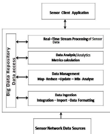
Figure 2: The layered architecture for the big-data analytics
