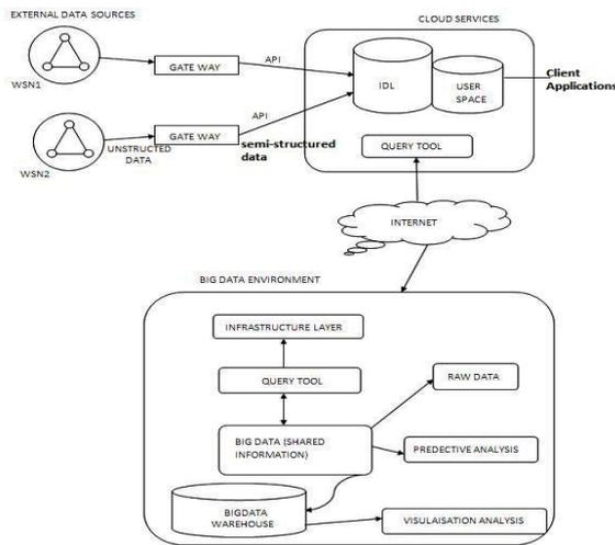
Figure 1: the big sensor Cloud data analytics and architecture.
