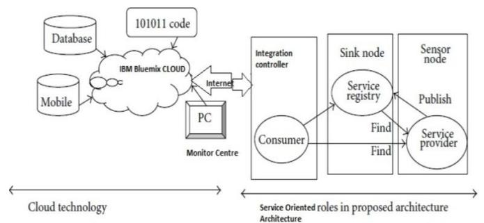
Figure 3: The SOSA extended to Cloud architecture.
