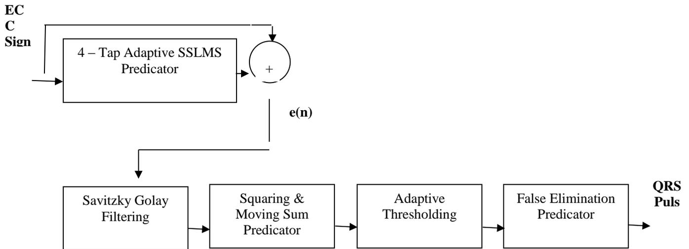
Figure 4: The QRS detection block diagram
