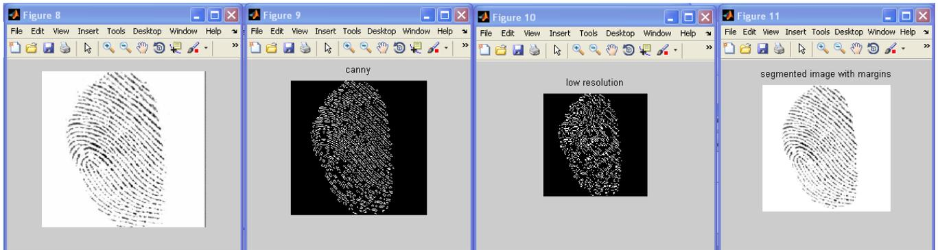
Figure 8: a) to d) Fingerprint preprocessing phases
