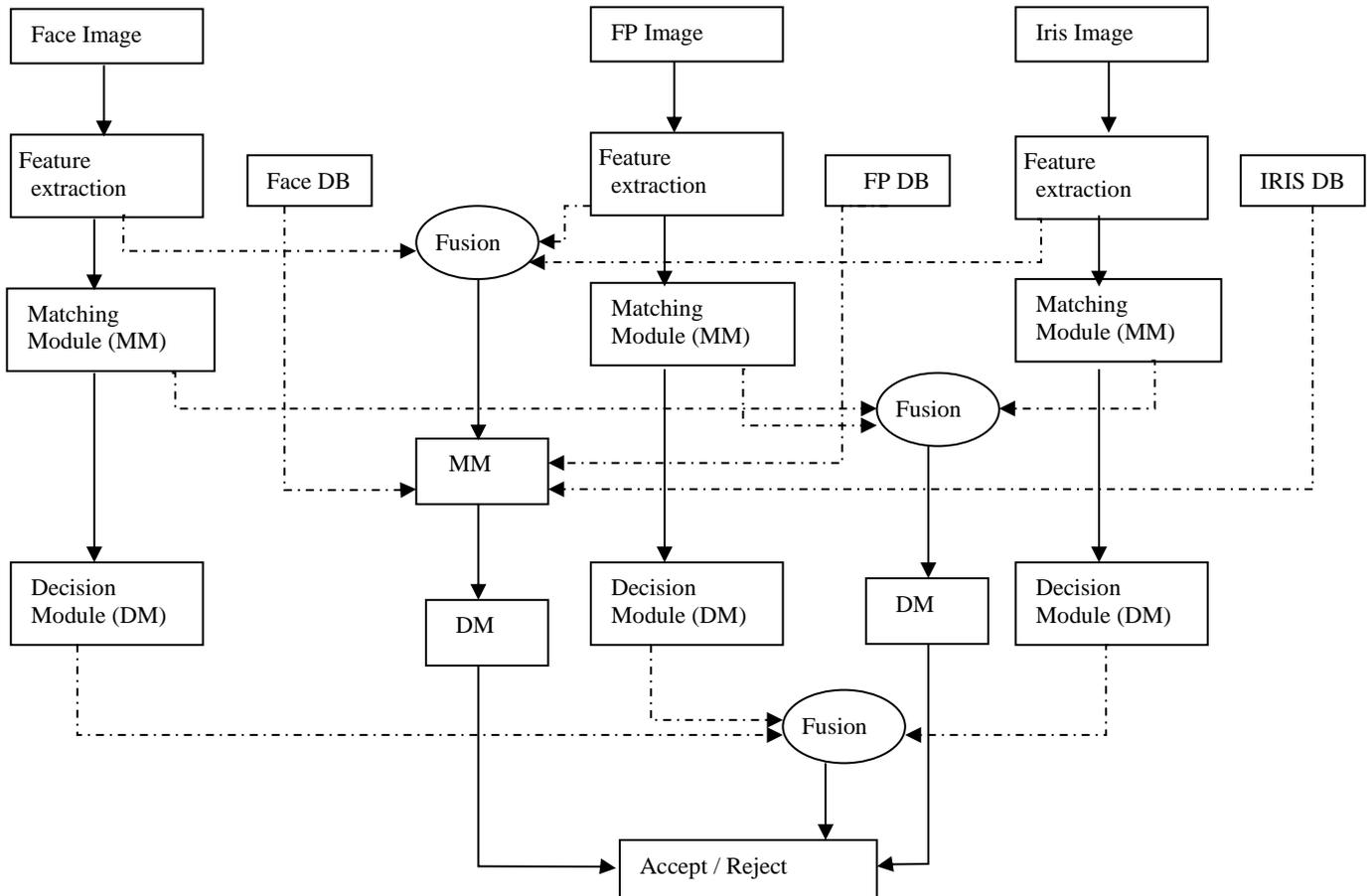
**Figure 1: Block Diagram showing different Levels of fusion used in Multimodal Biometric system**
