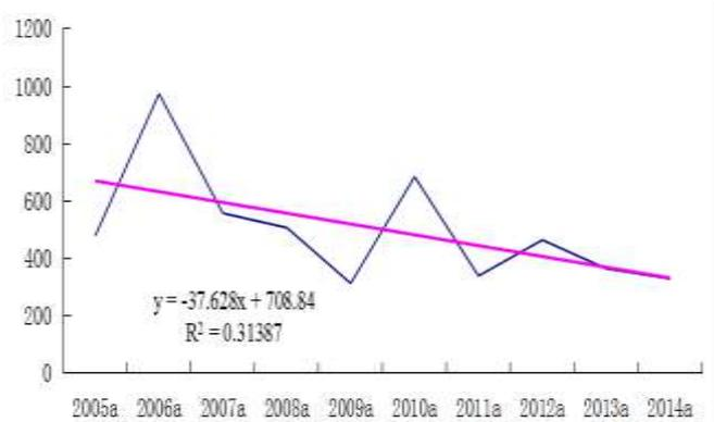
**Fig. 4: Linear regression of the sediment input of the reservoir area**
