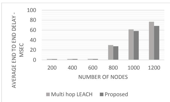
Figure 2: Average End to End Delay (sec)
