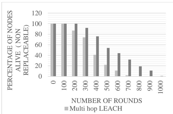
**Figure 4: Percentage of nodes alive (Non-replaceable)**
