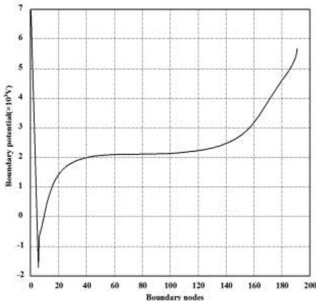
**Fig. 5: Boundary node potential of the four layer head model**
