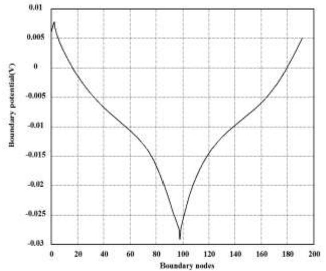
**Fig. 6: The boundary node potential of the four-layer model of the relative excitation mode**
