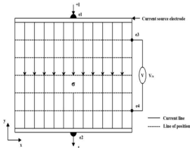
Fig. 1: The basic principle of the EIT system (rectangular conductor)
