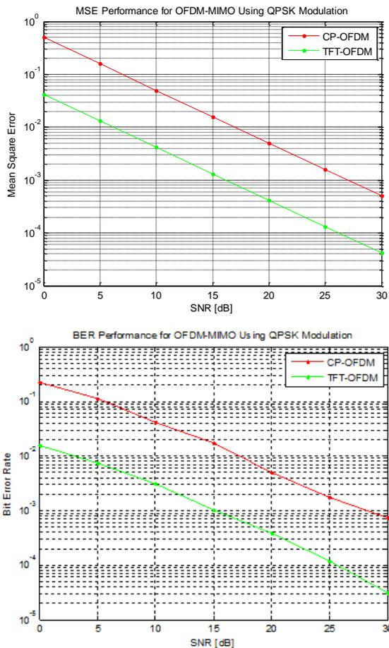
Figure 4: Performance Measure of TFT-OFDM with CP-OFDM. (a) MSE performance (b) BER performance.
