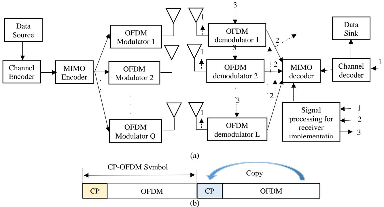
Figure 1: (a) MIMO-OFDM system; (b) Conventional CP OFDM
