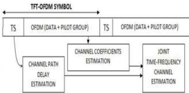
**Figure 3: Concept of Joint channel estimation on proposed TFFT-OFDM.**
