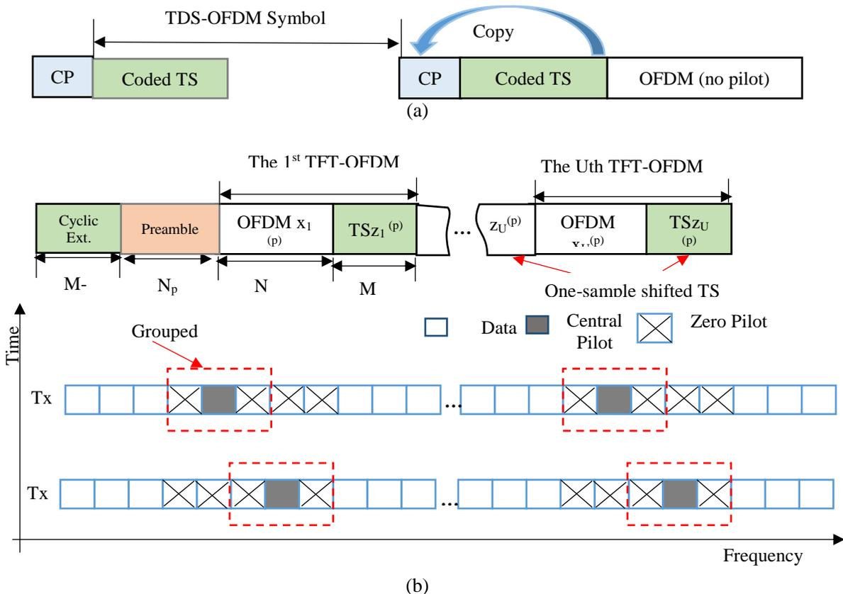
Figure 2: Time-frequency frame structure comparison of the MIMO systems on the basis of: a) Conventional TDS-OFDM; b) The proposed TFT-OFDM.
