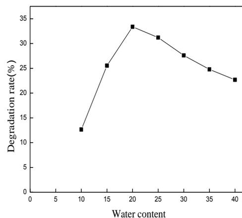
**Fig. 3: Effect of water content on the degradation of 2-chlorophenol**
