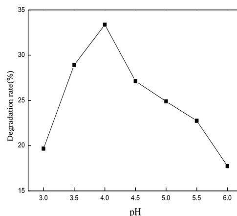
Fig. 4: Effect of pH on the degradation of 2-chlorophenol
