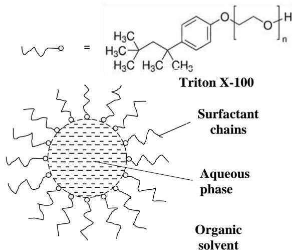
**Fig. 1: Diagrammatic sketch of Triton X-100 reverse micelles**
