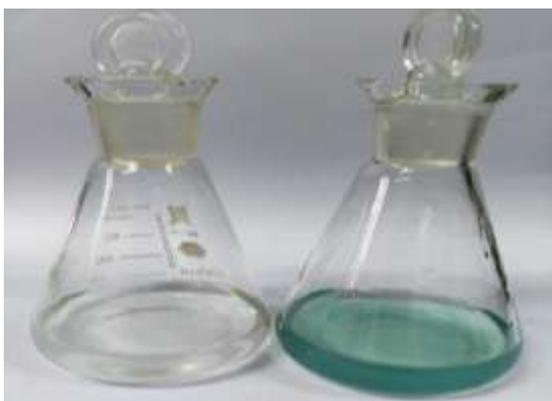
**Fig. 2: The left is laccase-containing reversed micelles, and the right is laccase / ABTS mediator-containing reversed micelles**
