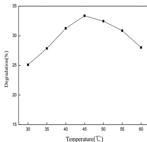
Fig. 5: Effect of temperature on the degradation of 2-chlorophenol
