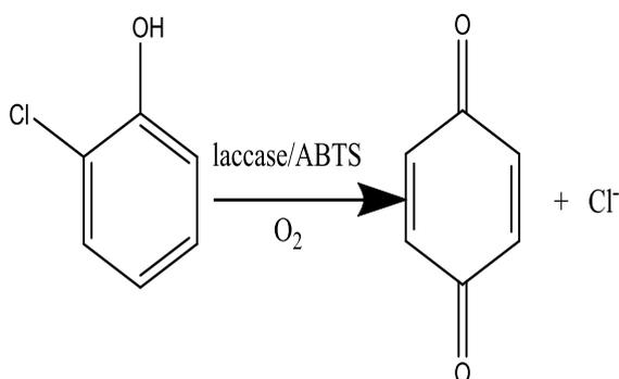
**Fig. 8: The pathways of 2-chlorophenol oxidation degradation**
