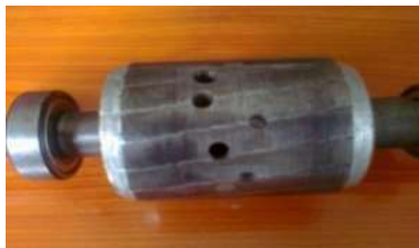
Figure 3: Photographic view of broken rotor bar
