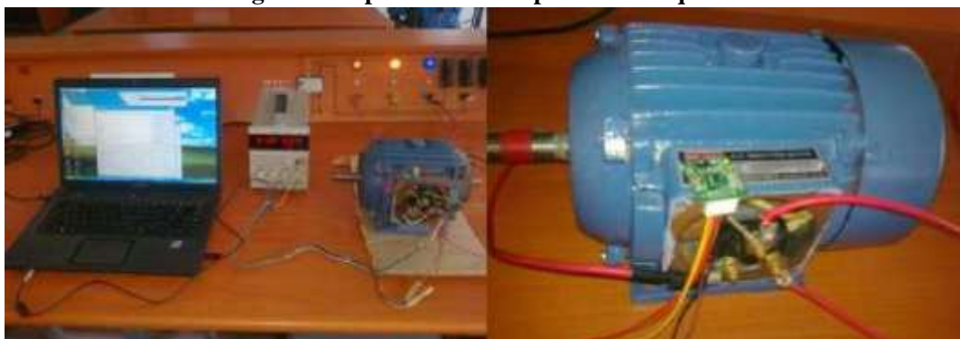
Figure 5: Photographic view of Experimental Setup and Accelerometer
